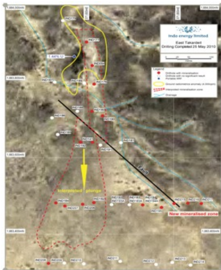
Figure 2: Showing Takardeit East drill holes, XRF readings and radiometric anomaly Carboniferous Drill Targets - Summary
